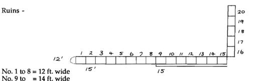
Casements 3 ft. x 1'6" - glass fixed with groove with strip nailed on, not made to open - a 5/8" rabbet (groove) formed by a 5/8" strip nailed on. No. 15 is 13 ft. wide.
