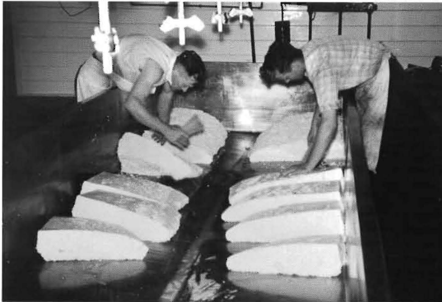
Cutting the curd and letting the whey drain out.
