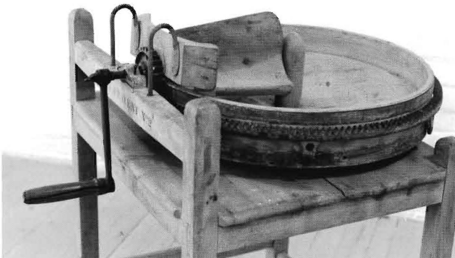
After the butter was churned, buttermilk was worked out using either pats or this type of mechanical butterworker. ( John Leeming photo, courtesy Dick Capple )
